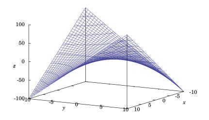
**Figure 2.5.1** f(x, y) = xy, saddle point at (0,0)
